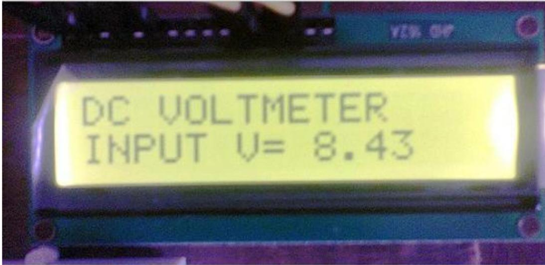
As you may be aware or are learning as we go along, the Arduino's analogue inputs can be used to measure DC voltage between 0 and 5V (when using the standard 5V analogue reference voltage) and this range can be increased by using two resistors to create a voltage divider. The voltage divider decreases the voltage being measured to within the range of the Arduino analogue inputs. Code in the Arduino sketch is then used to compute the actual voltage being measured.
