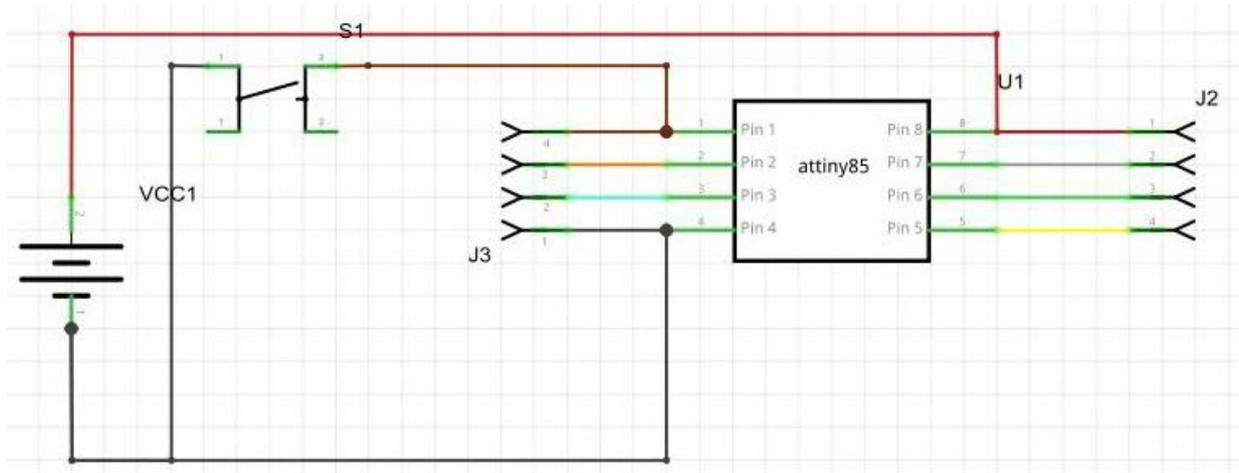
On my prototype I used a piece of Vero Board 11 rows by 21 holes, some male header pins, some female header sockets (so we can use the Attiny once programmed), a reset switch, a 10uF capacitor(required by the Uno for reset)
