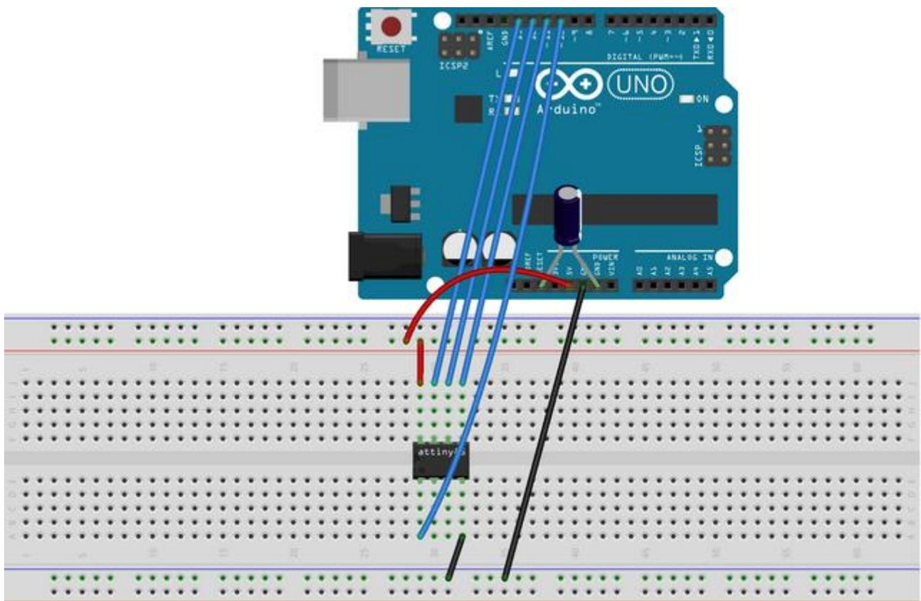
Pins are connected as follows, Gnd to pin 4, +5V to pin 8, Pin13 on Uno to pin 7, Pin12 on Uno to pin 6, Pin11 on Uno to pin 5, Pin10 on Uno to pin 1(Reset). Pin 9 goes through a 220R resistor and LED to ground as a heartbeat to show that it is being programmed.
