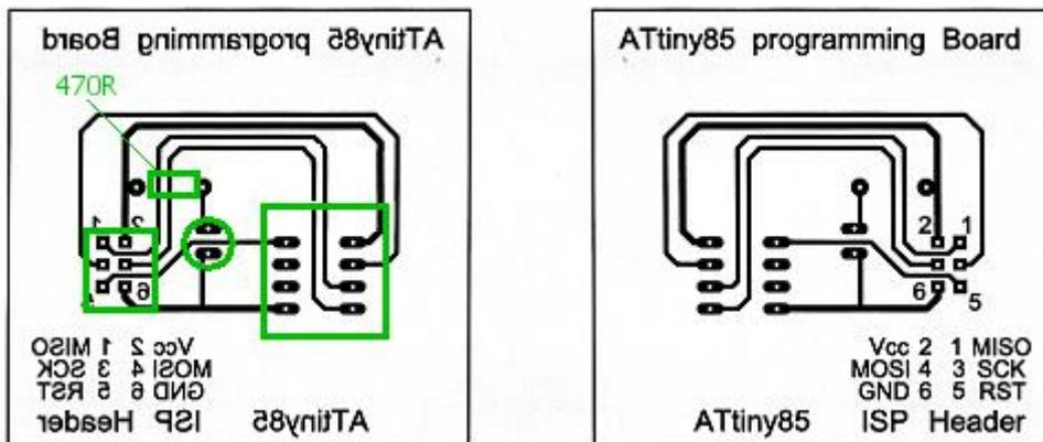
All that is required is a 470R resistor, an LED, an IC socket and a 6way ISP header. This programming board can be used with a USBASP programmer or the Arduino ISP pins.
