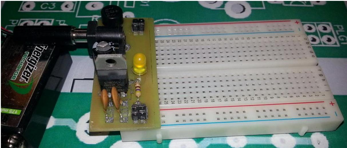
The circuit diagram for this little project shows the standard configuration for the LM7805, a 1A – 5V linear regulator. All we have done is to design a simple layout on PCB, add a rectifier so that you can use either a DC or AC 12V adapter and feel safe that you won't let the smoke out of any projects.
