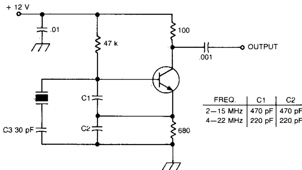
Using the values for the 4-22MHz option in the diagram above I have found pretty accurate readings to within the specified ratings for most crystals under test. My test oscillator actually runs up to just over 30MHz and is used quite often as a reference oscillator and not just to test crystals. An important fact to remember here is that in effect,
