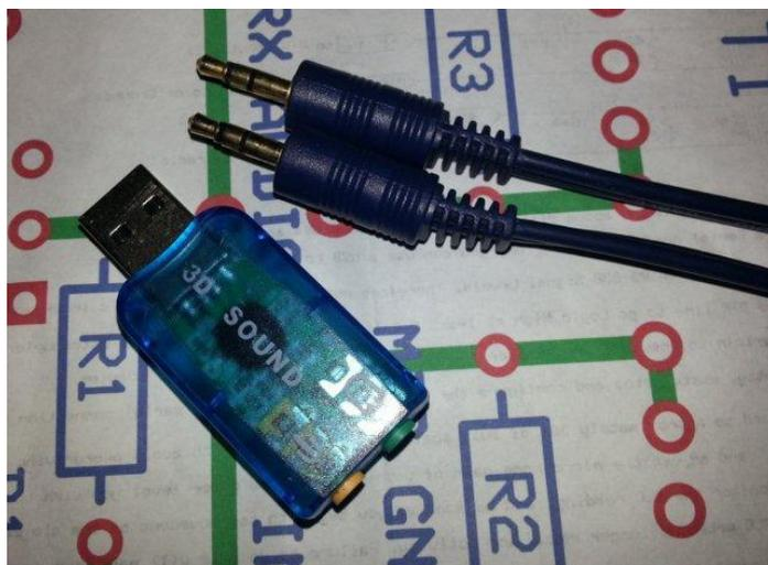
Removing the sound card from the casing, desoldering the audio sockets for line input and speaker output was simple enough. Connecting the digital interface to the soundcard input and output was just as easy, remembering that only one channel was required. I cut a slot in the side of the enclosure to allow the USB port to protrude once mounted to the inside of the enclosure and for the standard USB extension cable to fit.
