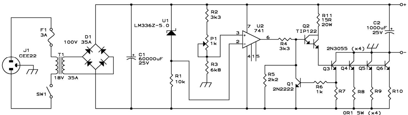
This power supply delivers a highly regulated 13.8V, adjustable over a moderate range, at a continuous current of up to 20A. It is current-limited to approximately 25A, and short circuit protected for as long as the heat sink can keep the transistors cool enough. It is probably the simplest design that can accomplish this.
