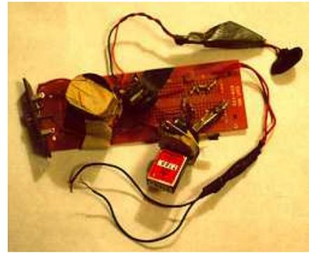
A **very** quick and easy way to get on the air is to build a "Michigan Mighty Mite" CW transmitter for 160, 80, 40 or 30 meters originated by Ed Knoll, W3FQJ and developed by Tom Jurgens, KY8I. It can't get simpler than this! I made my very first QSOs with a 40-meter version (photo). It has very few parts, costs almost nothing, and **it works!**
