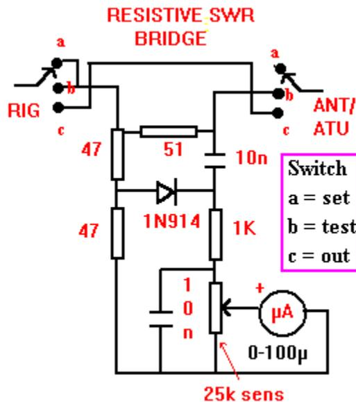
The bridge shown is popular with QRPers. There is no setting up to do and the circuit need not be laid out symmetrically as with other designs. I used a tiny meter bought from Kanga (UK), only about 0.75" x 1", but any meter less than 1 mA should do OK. Although a 3-way switch is shown, a DPDT toggle can be used, as once the bridge is calibrated, only an 'in/out' switch is required.
