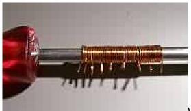
• Wind 6 turns x - 2 connections on your switch (in this project a 10-posistion rotary switch is used, being 8 times 6 = 48 + 4 + 3 = 55 turns) over a 7mm screwdriver (or simular obkject hi) and make a tap every connection. Solder each tap.
