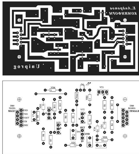
Please note, that R12 is omitted on the PCB, Rind resistor and a LED are added between the DA1 output and the ground to indicate the power. You can omit R12, Rind and a LED, the circuit will work. Some words are in Russian, the most significant words are translated. The recommended value of Rind is 4.3 kOhm to minimize the current consumption.
