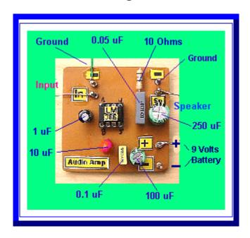
The LM386 IC has been designed to work with low voltages...between 4 to 15 volts. The current taken from the power source or the batteries when standing by, is also quite small, something around 3 mA's. If you add to these qualities the possibility of changing the amplification power, you realize that the LM386 chip is an attractive circuit to work with.
